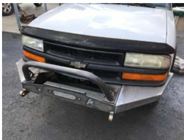
STEP 5 - INSTALL BULL BAR WITH HARDWARE SHOWN ON SHEET 1.
