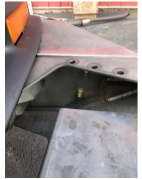
STEP 4 - INSTALL BUMPER END SECTIONS WITH HARDWARE SHOWN ON SHEET 1 AND ADJUST ENDS AND CENTER BEFORE TIGHTENING.
