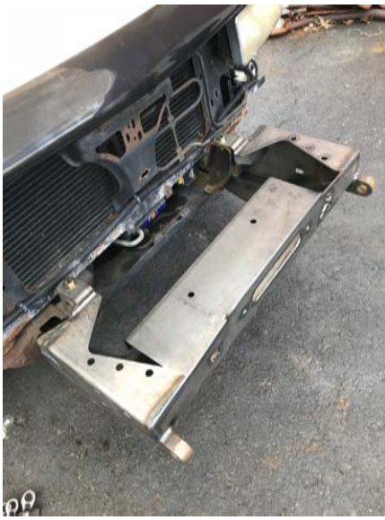
STEP 3 - SLIDE BUMPER CENTER SECTION ONTO FRAME RAILS AND MOUNT WITH HARDWARE SHOWN ON SHEET 1.
