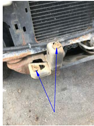
STEP 2 - REMOVE CLIPS SHOWN IN PICTURES ABOVE.
